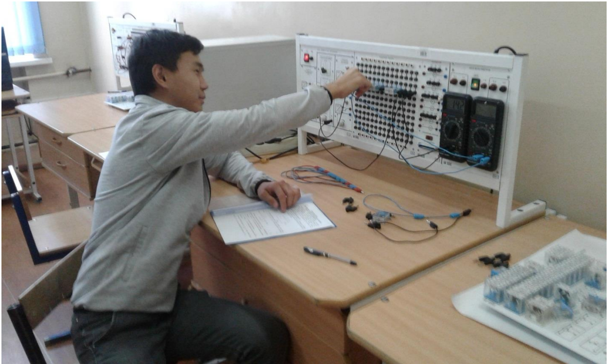
Figure 18. Educational and laboratory stand on the theory of electrical circuits
