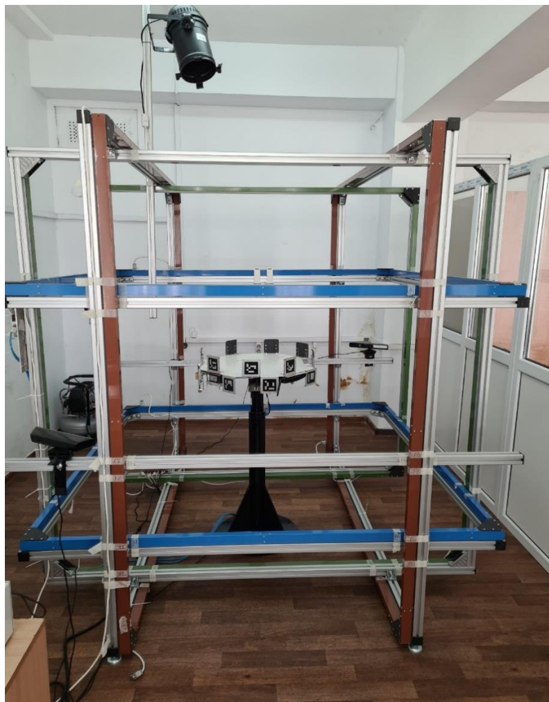
Figure 5. Stand for simulation of relative motion and testing of orientation and stabilization systems of SX-025 nanosatellites
