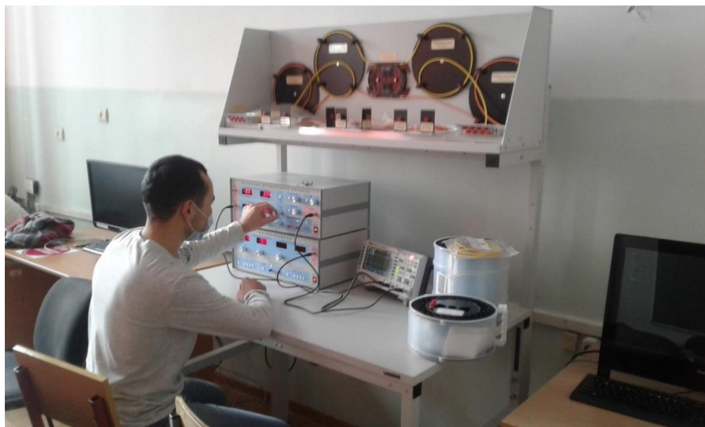
Figure 11. Educational laboratory installation "Optical linear path model"
